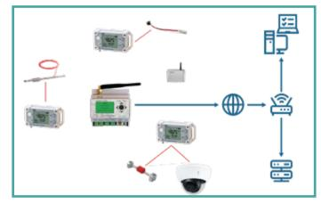
Static Monitoring: for pillars and supports, beams through joint gauges, clinometers, extension gauges. It allows for the evaluation of the static behavior of critical components of works to monitor their conditions while operating and highlighting the consequences of decay and/or deterioration.
